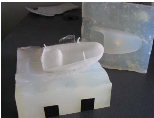
Figure 2. Silicon rubber mold and part obtain by Vacuum casting process, source of [1]
